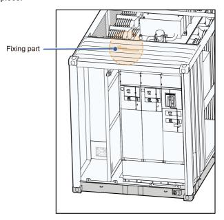
\* For some products, before removing the fixing piece, it is needed to remove the side baffle plate at the upper left of the RMU. The location of the plate is shown in the figure below.
