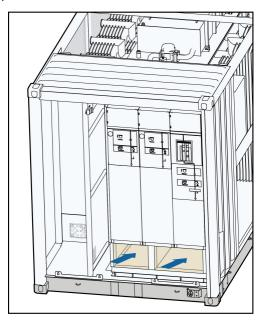
**Step 4** Unscrew the M5×16 cross-recessed hexagon bolt assemblies to remove the bottom sealing plate of the RMU.
